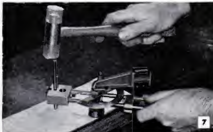
Above, a protractor is fitted into a slot cut in the head of the pivot bolt as in detail on opposite page. Protractor is held in place with setscrew. Below, circle tool can be attached to work or bench top. Works on full circle or any size segment
